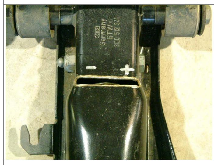
Once the slot has been completed, spray the slot with some type of anti-rust corrosion resistance spray.
