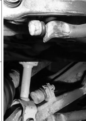
4 Loosen (but do NOT remove) the bolt that attaches the ARB link to the ARB.
