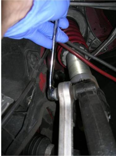
7 Remove bolts that connect damper fork to lower link and damper. Use spreader (Audi Tool # 3424 or equivalent) to remove fork from damper. Pull bearing housing down to gain enough clearance to remove fork.
