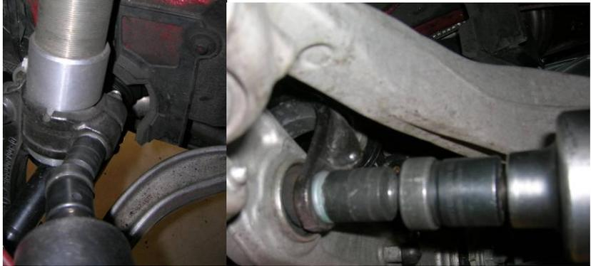
8 Perform these steps on both sides of the car and then open the front hood to reach the bolts that hold the upper mount.
