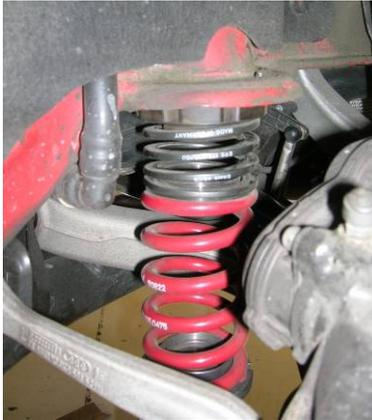
8 Install the OEM upper damper mount onto the STaSIS damper. Grab cylinder head with a wrench and tighten nylock nut to 37 ft-lbs.
