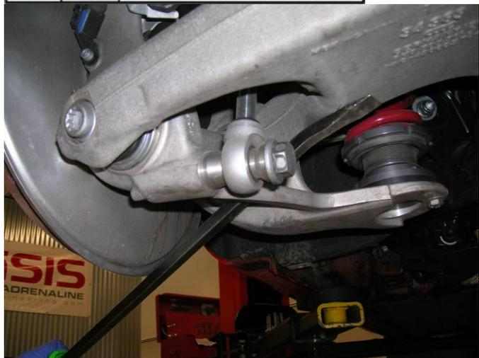
5 Remove the OEM lower rubber spring mount, it will not be reused.
