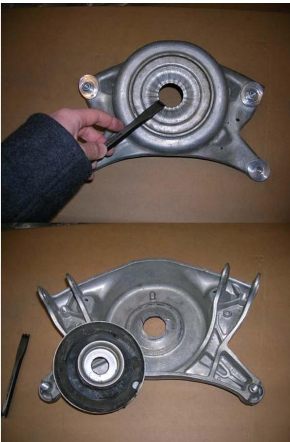
15 Install spring with delrin upper mount onto the STaSIS damper.
